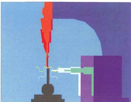
• 2-D OPERALOG software, enables the user to draw the part profile. It calculates the developed length, backgauge axes position, punch penetration, spring back and detects any possible collisions between piece part and the machine.
