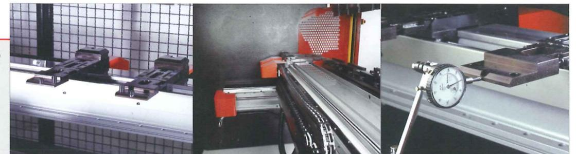
Bend accuracy is highly dependent upon the backgauge. Five, independent axes (X1, X2, R, Z1 and Z2) are driven by large recirculating ball screws.
