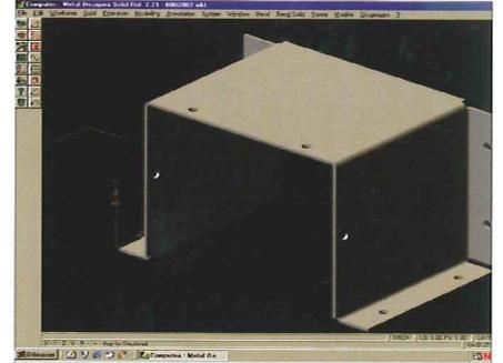
• A comprehensive bending software package, PBs permits bend simulation in a 3-D environment. Using PBs, you can prepare and test the program before going into actual production. By linking PBs to the Opérateur 2002 controller, the press brake can be freed from none productive tasks.
