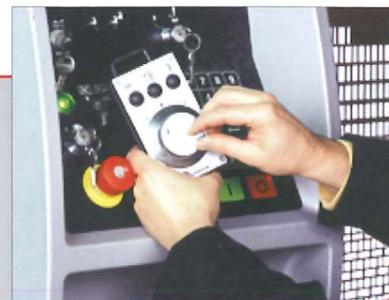
Ergonomic and robust, this new hand wheel-teaching device is a standard feature on all HFE press brakes. This unit allows the operator to individually control the upper beam movement ( Y1 and / or Y2) and all backgauge axes in order to carry out manual adjustments.
