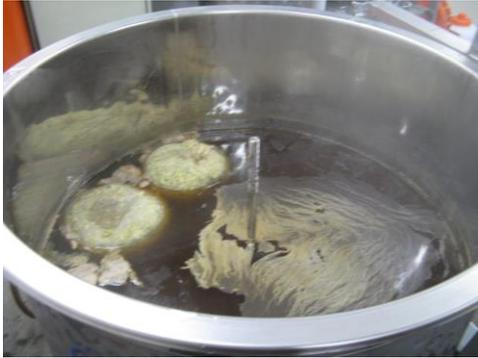
Continue by pressing the *Select* button in order to start the hops boiling process. Do not close the lid. Avoid the hops boiling over. Add the first batch of hops (200 g or 350 g or 700 g) 10 minutes after the boiling point has been reached. Do not close the lid during the hops boiling process either. Steam must be able to escape. Top up evaporated water quantity or adjust original wort. Ten minutes before the brewing process is finished, add the last batch of hops (100 g or 150 g or 300 g).
