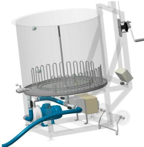
Immediately after the brewing process, it is strongly recommended to place the Braumeister into its cleaning position (see illustration on the left-hand side). Use water to dilute the trub substances and pump out the residue. Observe the correct position of the valve.
