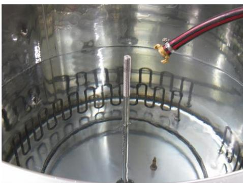
Add 230 L/575 L/ 1200 L brewing water – to the upper marking on the tie rod or filling level indicator. Follow the instructions of the brew control by pressing *Select*, acknowledging that water has been added. Venting of the pump takes place automatically, followed by heating up to the programmed mashing-in temperature.
