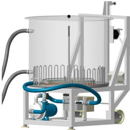
Connect the hoses and position the valves as seen in the illustration on the left-hand side. Selecting a low pump speed (set to 6-8) ensures a consistent rotation of the wort inside the vessel. Caution: The pump will only restart again at 86°C. The consistent rotation will also optimise the cooling process. Cooling the liquid from 100°C to approx. 25°C (if using ice-cold water) requires approx. 50 min/120 min.
