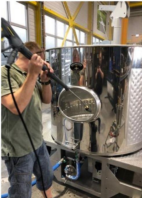
Best cleaning results can be achieved by a high pressure cleaner. On the Braumeister 1000 L it's possible to remove a manhole in front of the vessel for a better accessibility for cleaning, inspection and service.
