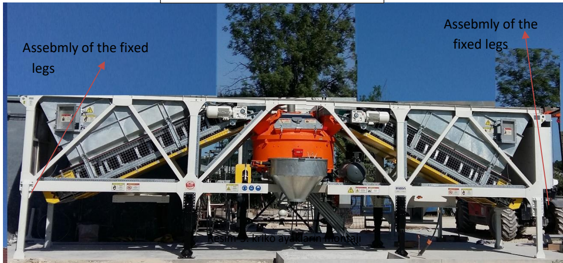
Picture-4: Assebmly of the fixed legs
